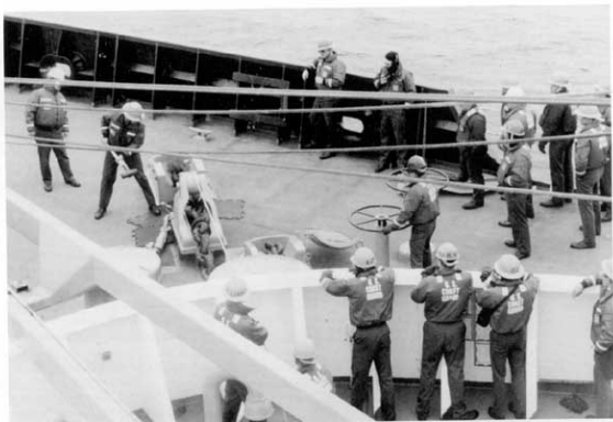
Deck Force hard at work lowering the starboard 9,000 lb. Navy Stockless anchor.
