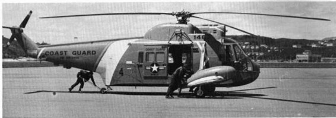
There are 3 ways of starting it, ship's power, helo's batteries, and the push start
