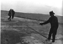
It was often necessary to salt the flight deck before flight operations because of ice build-up.
