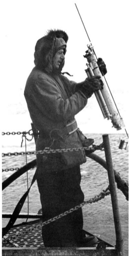
Nansen bottles were used to collect water samples at various depths. The bottles also had reversing thermometers to record the water temperature at the depth collected.
