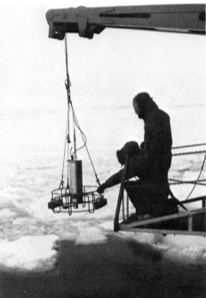
An electronic sensor which is used to record changes of salinity, temperature and depth as it is lowered through the water. The data is collected automatically on chart paper.
