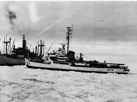
After chopping out mooring site and having cargo ship follow astern, Eastwind holds USNS Towle against ice ledge while crew members on ice secure mooring lines.
