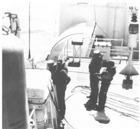
Tending the T & D line (telephone and distance line) during underway replenishment at sea operations
