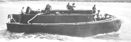
CG-40362-F is 40-ft of boat loaded with the latest fire-fighting equipment. Here swaths water around her with foam.
