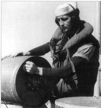
Left: A Coast Guardsman sets the detonating depth on a depth charge aboard the USS PC-556, Oct. 8, 1942.
