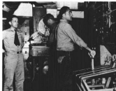
Answering bells on the main control board
