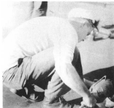
Scraping the deck before painting
